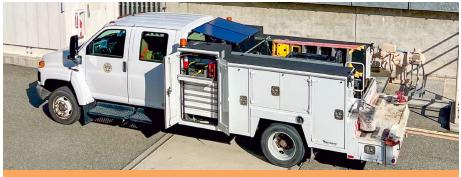
Solar-powered, truck-mounted generator
