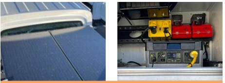
Components of the solar generator fitted to a work truck. From left to right: battery inverter in the storage compartment, a close up of the Yeti battery inverter, and two 200-Watt solar panels on the back of the truck.
