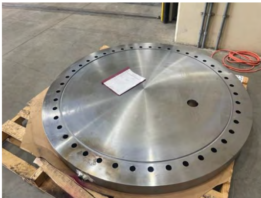
Machined top flange (left) and application of completed coating on top flange (right)
