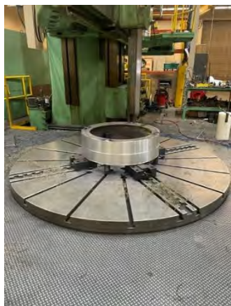
Machining of lower section (left) and finished machining of lower section in process (right)
