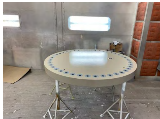
Machined top flange (left) and application of completed coating on top flange (right)
