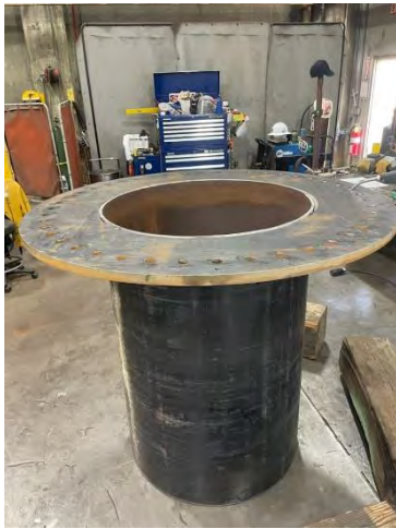
Fabrication of middle flange (left) and ring (middle) and fabricated and machined 96-inch-long segment (right)
