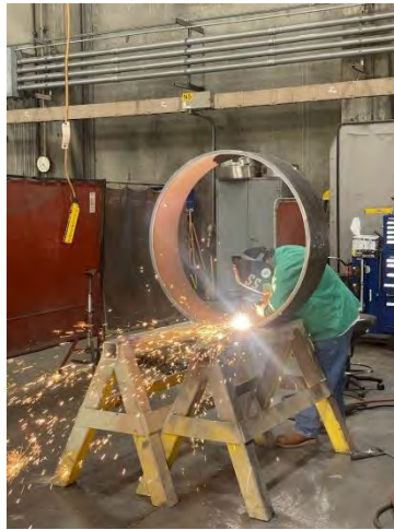
Fabrication of middle flange (left) and ring (middle) and fabricated and machined 96-inch-long segment (right)
