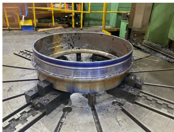
Machining of lower section (left) and finished machining of lower section in process (right)
